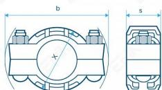
A536 Gr. 65-45-12 / Gr. E (EPDM), A536 Gr. 65-45-12 / Gr. E (EPDM) hot dip galv., A536 Gr. 65-45-12 / Gr. T (Nitrile), A536 Gr. 65-45-12 / Gr. T (Nitrile) hot dip galv., A395 Gr. 65-45-15 / Gr. E (EPDM), A395 Gr. 65-45-15 / Gr. E (EPDM) hot dip galv., A395 Gr. 65-45-15 / Gr. T (Nitrile), A395 Gr. 65-45-15 / Gr. T (Nitrile) hot dip galv.
